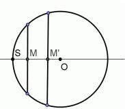
Let us consider a thin slice of sphere, spherical cap between the points M and M'. We set SM = x and  $MM' = \tau$ . This slice has its center of gravity on the segment MM'.
