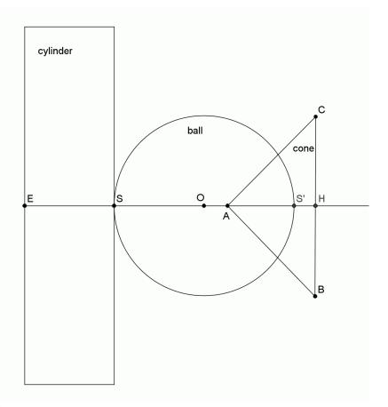
The second disk generates a cone, since the radius increases with the distance. This cone has its center of gravity at S', point symmetric to S with respect to O, (so SS' = 2r).
