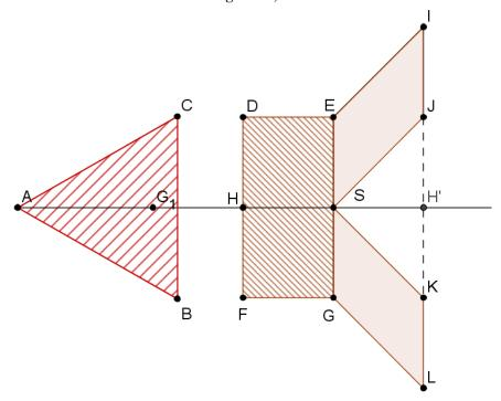
In this picture, the cone ABC, with summit at A, height r, base BC of radius r, plus the cylinder DEFG, height HS=r, radius HD=HF=r, is in equilibrium around S with the piece of cone generated by the rotation of SEIJ: this is the cone IHL, with summit at H, truncated at E, minus the cone JSK. We have ES=IJ=SH'=r.
