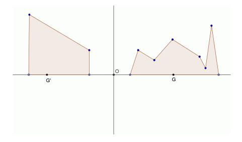
We discretize our original solid in small cylinders; it does not matter whether these cylinders have equal thickness or not). Then we can put these cylinders in decreasing order of radii on the left side of the axis: we clearly have a solid with same volume, which is decreasing in the sense we explained.
