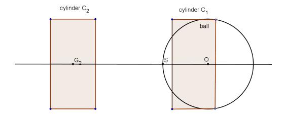
On this picture, the red cylinder  $C_2$  (left) is in equilibrium around S with the ball and the red cylinder  $C_1$  (right).
